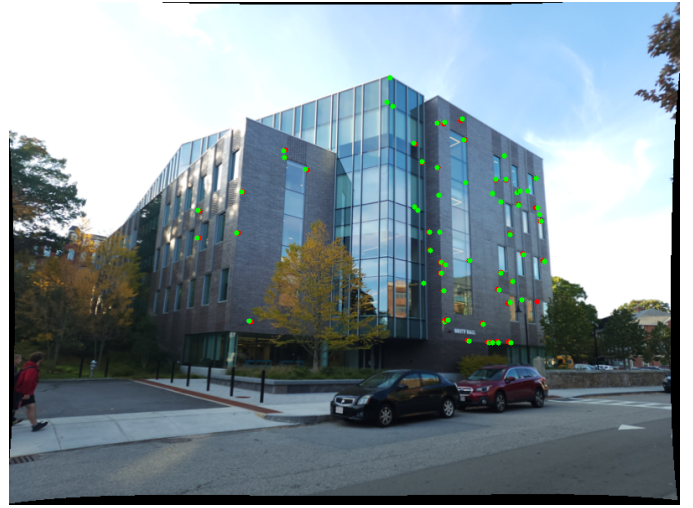
Fig. 10. Nonlinear PnP Reprojection for Camera 4
