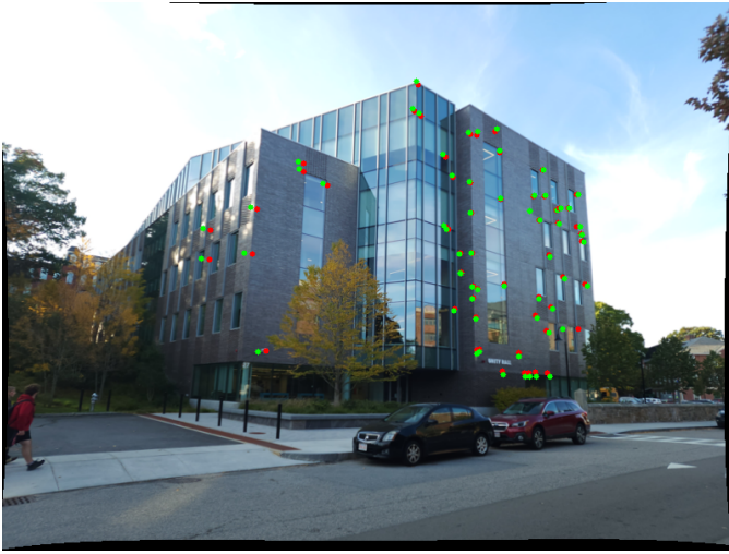
Fig. 9. Linear PnP Reprojection for Camera 4
